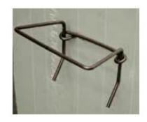
Cast-In Place Brick Tie and Pintle. — Enables solid anchorage of veneer masonry through exterior foam to concrete core; tested to meet ASTM D754 (USA) and CSA-A370 (CAN) std. requirements for masonry anchors.
